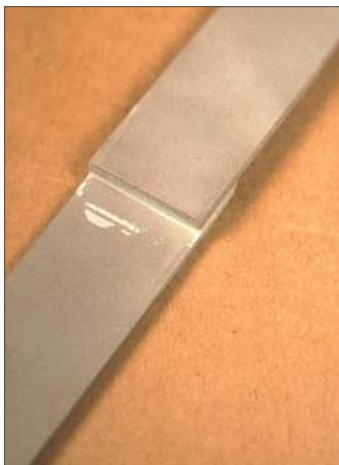
Overlap shear test; two steel.
