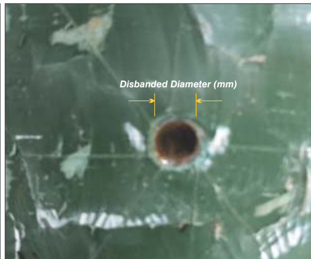
CD test panel after test is completed.
