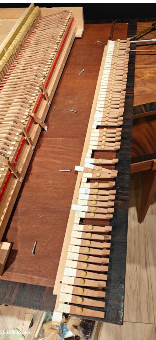
THESE ARE LEATHER PADS WHICH CAN BE ADJUSTED TO FINE-TUNE THE ACTION OF THE KEYS
