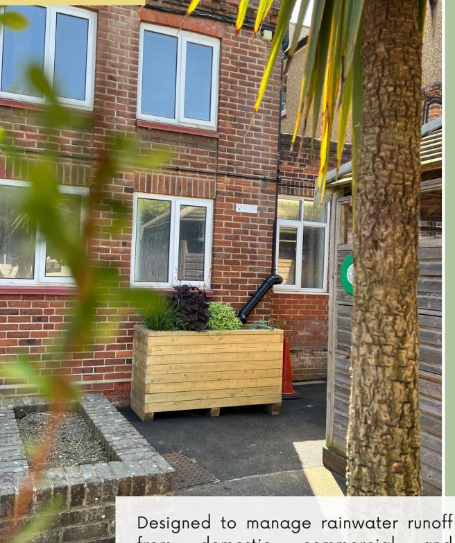
Designed to manage rainwater runoff from domestic, commercial and industrial roofs, they collect runoff and function as a rain garden within a planter, allowing for sustainable stormwater management.
