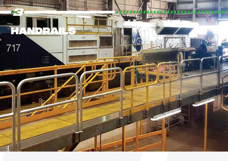
Our design, engineering and manufacture of handrailing for locomotives, wagons and rail workshops have increased safety as years and legislation has passed. All of our handrails are designed for full certification and compliance with Australian Standards.
