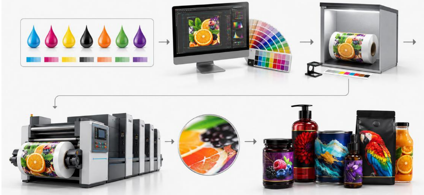
simple ECG workflow visual — CMYKOGV ink set, prepress/profile, proofing, press and finished labels.
