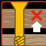
Partially Threaded Stops The Timber Jacking
