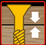
Dual Angle Thread Designed For Superior Hold
