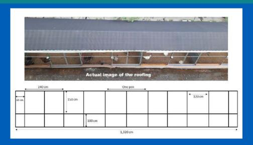
The total length of the frame for roofing for the housing is 1,320cm. An extra 60cm on both sides is added on 1,200cm to come up with such length. On the 150cm length, it will be the bending part. It will be toward the back/rear side of the housing. Wield the supporting frame on the bending length to support the trusses of the roofing. These measurements are shown in the above figure.
