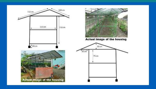
For the side view of the housing, it is presented in the figure in this page. The total height from the footing to the topmost of the housing is 200cm. The width is 120cm, and the height from the truss to the supporting frame is 75cm. The height from the supporting structure to the base is 75cm, as well. The width of the roofing trusses is 250cm. More measurement is shown in this figure.
