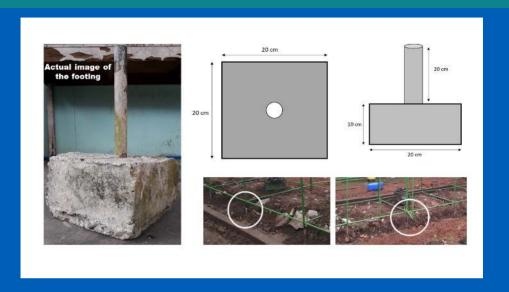
Moreover, the housing should have a footing that will be buried in the ground (figure in this page). It has a dimension of 20cm in a square with a 10cm thickness. It has embedded with  $^{3}\!\!/_{4}$  GI pipes having a height of 20cm, where an extra length of  $^{1}\!\!/_{2}$  GI pipes from the frame (as the post) will be inserted and partially welded.
