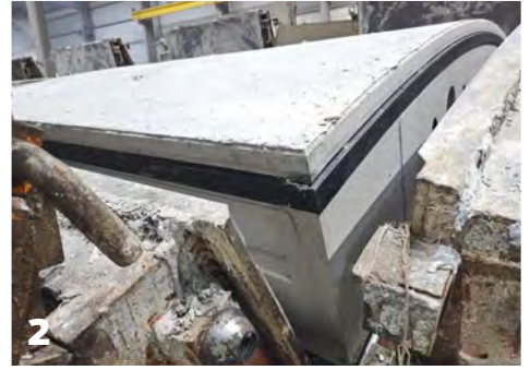
[1]: The mold is oiled for the easy removal of the tunnel segment. [2]: After the initial cure, the mold is opened so the tunnel segment can be removed.
