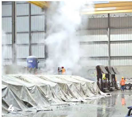
[4,5]: The molds are covered and the tunnel segments cure for several hours before removal.
