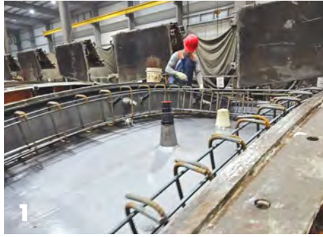
[1]: The mold is oiled for the easy removal of the tunnel segment. [2]: After the initial cure, the mold is opened so the tunnel segment can be removed.
