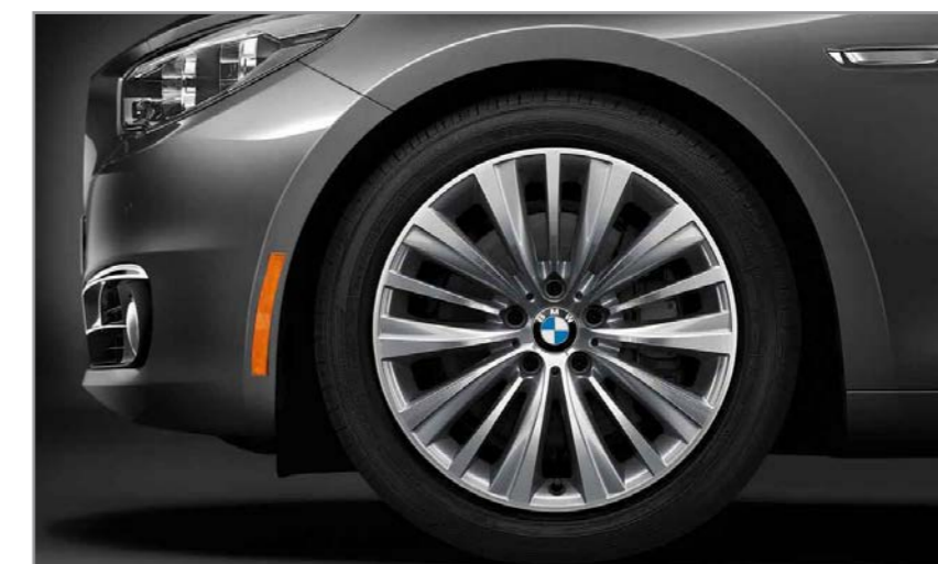
Multi-spoke light alloy wheels (Style 458) 19 x 8.5 front and rear; and 245/45 front and rear run-flat all-season tires 1
