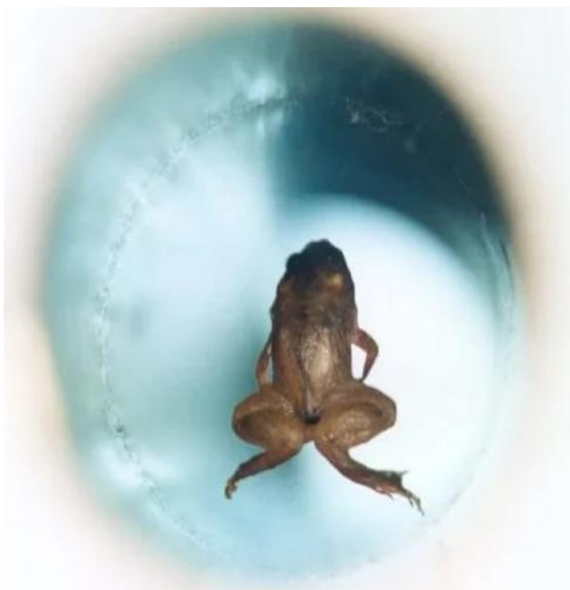
A live frog levitates inside the vertical bore of a Bitter solenoid in a magnetic field at the Nijmegen High Field Magnet Laboratory.
