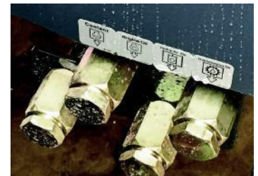
Autolube is a standard feature on the Taylor T-1023. All pressure taps and site gauges are easily accessible. Fluid drains provide environmentally friendly drainage capability and are grouped together for convenient serviceability.
