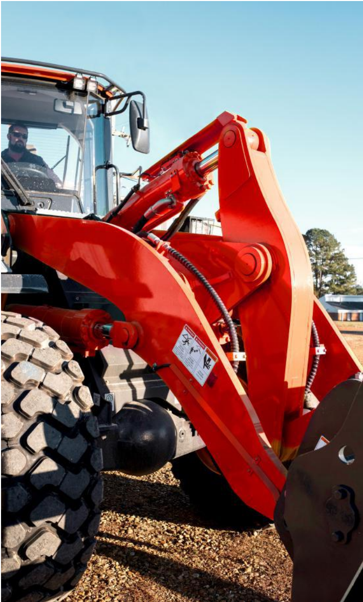
The Taylor T-1023 features optimized Z-Bar geometry that positions the bucket closer to the tires, achieving high bucket breakout forces with maximum rollback. The hydraulic quick coupler attachment adds versatility to Z-Bar machines, allowing use of multiple tools to suit the job-site needs.
