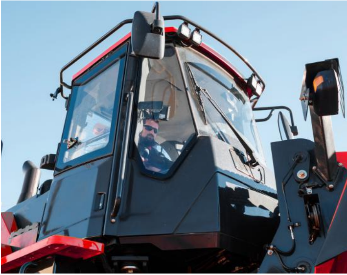
The Taylor T-1023 has been designed to offer optimized visibility. A panoramic view cab with curved front glass has been paired with well-positioned lift arms to allow the operator a clear line of sight to the attachment at ground level.
