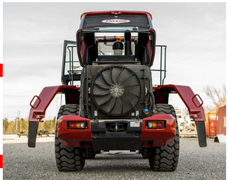
The rear full fenders swing out for easy access to the engine compartment. The electrically actuated, wide opening fiberglass hood of the Taylor T-1023 gives you easy access to the engine and its easy-to-reach service points. The radiator also swings out for ease of service.
