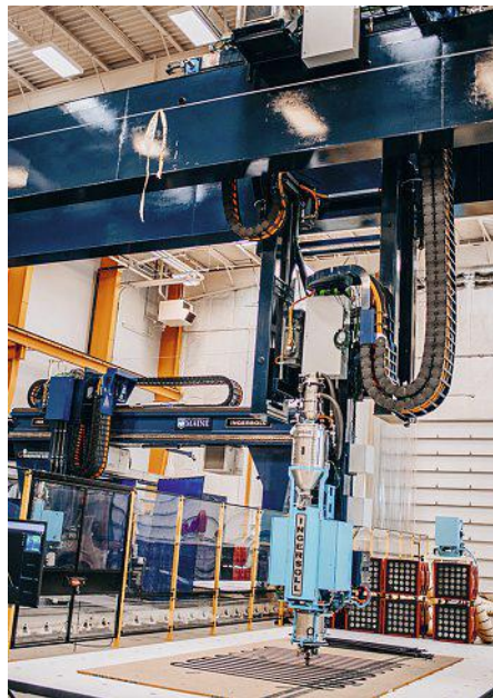
Above The gantry-mounted system at the University of Maine's Advanced Structures and Composites Center is capable of carrying out multiple construction manufacturing processes, not just 3D printing.
