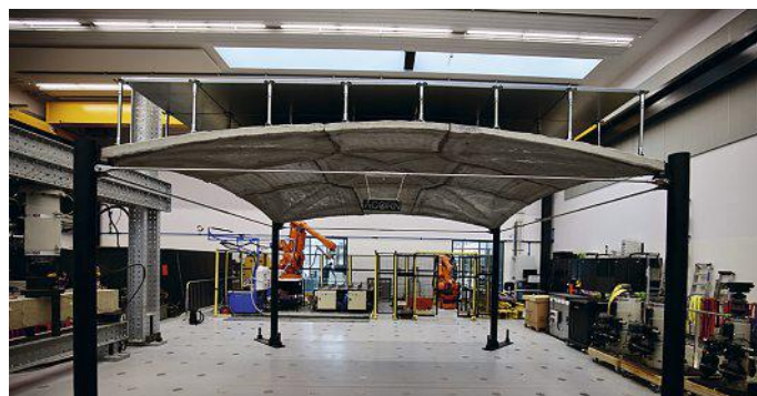
Left Researchers at the University of Bath made a robot-manufactured 'thin shell' vaulted floor slab with 60 per cent less embodied carbon than an equivalent flat slab.
