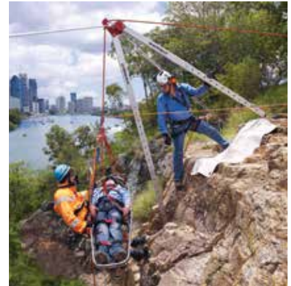
(top) Gin Pole / Monopod (bottom) Offset A-Frame
