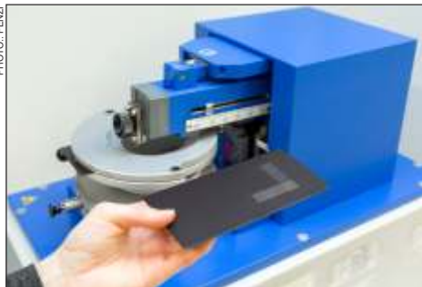
Cross-cut tests show that the adhesive properties of SILRES® M 51 E are similar to those of high-temperature paints and coatings formulated with solvent-based silicone resin binders.
