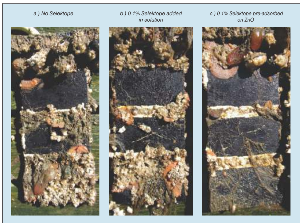
Figure 3. Panels with foul release topcoat after 419 days submersion in the sea outside of Tjärnö (west coast of Sweden). The panels are divided in three sections where the top sections were left undamaged, the middle sections have a cross cut with knife and the surface of bottom sections were roughened with sandpaper. The topcoats contain the following additive, from left to right a) no additive, b) 0.1 weight% Selektepe added as solution and c) 0.1 weight % Selektepe added as a powder additive consisting of 10 weight % Selektepe adsorbed on the surface of ZnO.
