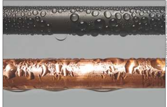
Copper steam condenser pipes coated with F-DLC (top) and without a coating (bottom). The F-DLC coating allows the condensed water to form into droplets rather than a thin film covering the pipe.
