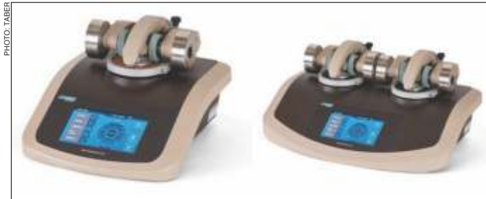
The single platform Taber Rotary Platform Abrasion Tester Model 1700 and the dual platform Model 1750.
