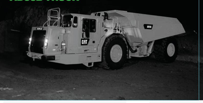
A platform designed for the safe, certified and compliant access to the to the tray of the AD55B Underground Dump Truck.
