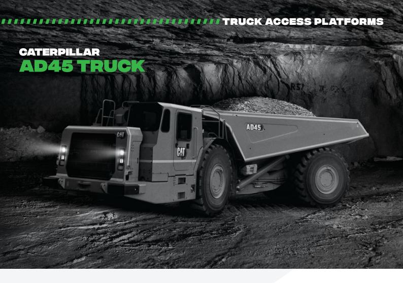
A safe, certified and compliant access platform designed and engineered to access the tray on the AD45 Underground Dump Truck
