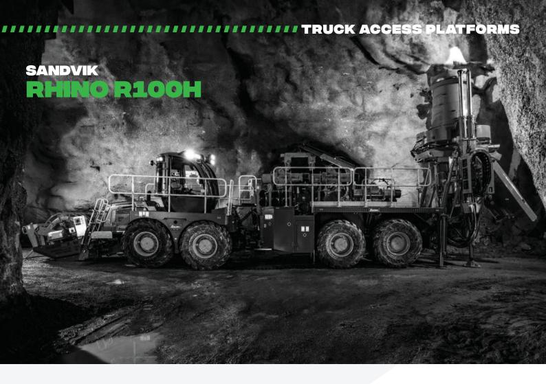
Access and walkway steps made to make maintenance safer and more efficient on the Sandvik Rhino R100H. Designed and built to withstand the harshest underground mining environments.
