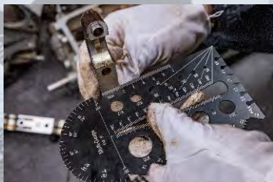
Gage Leg Quick-Check Perpendicularity
