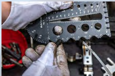
Pitch Size Measure the Thread
