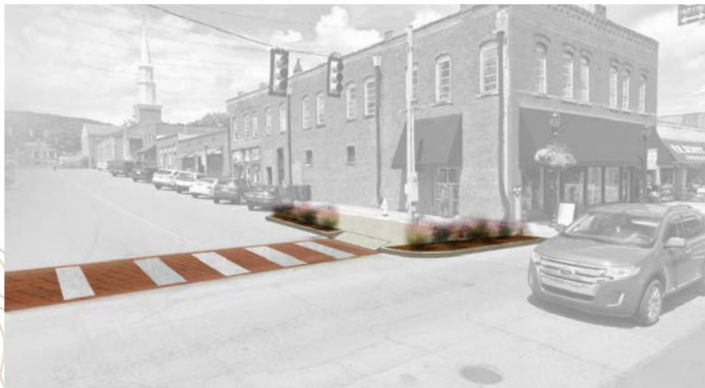
Proposed curb extensions and high-vis crosswalks on Gault Ave at 1st Ave
