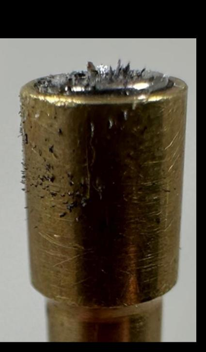
FOD refers to any material that is not part of the engine, such as dust and debris from maintenance work and oil servicing
