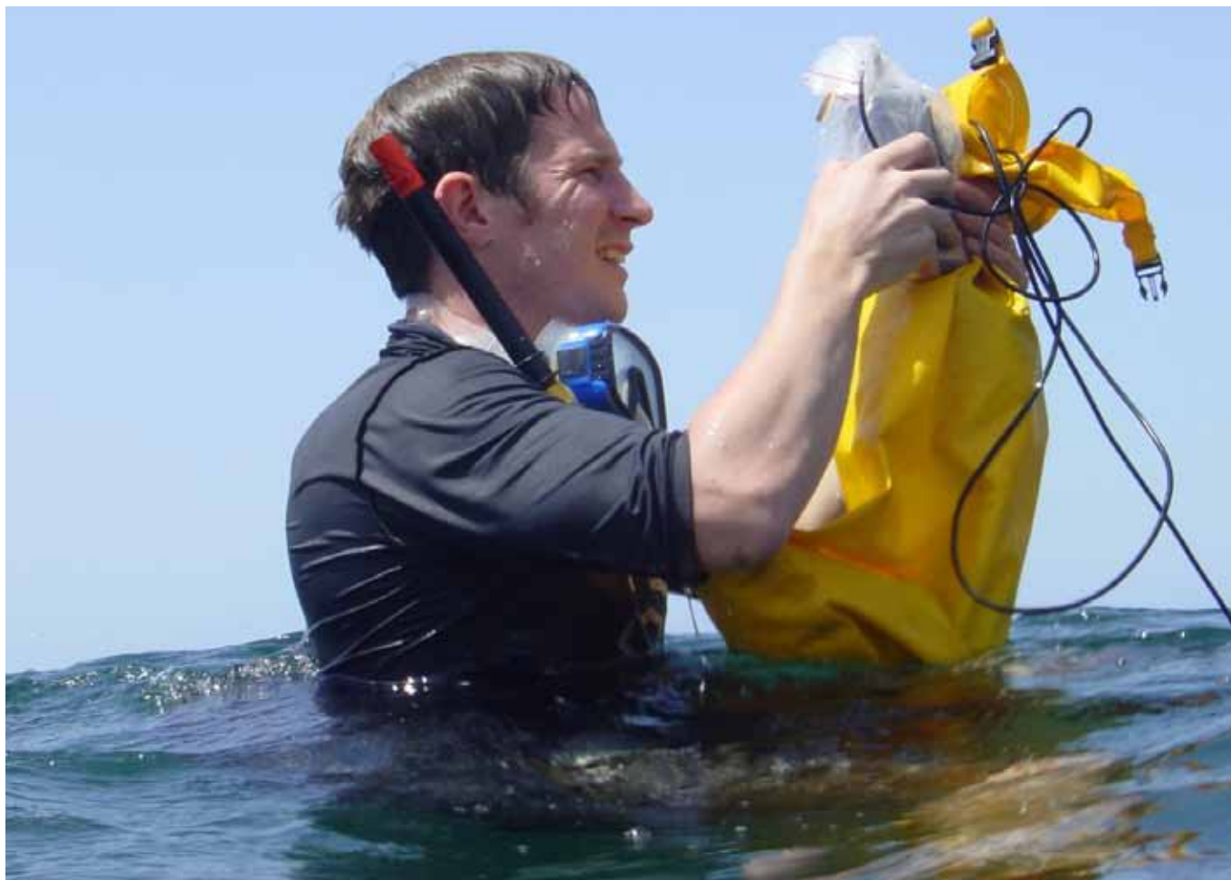
The sounds of coral reefs can be recorded in the field using an underwater microphone known as a hydrophone. Apart from the hydrophone, the rest of the recording equipment is far from waterproof. Recording off Hoga Island (2007), by Dr Stephen Simpson.
