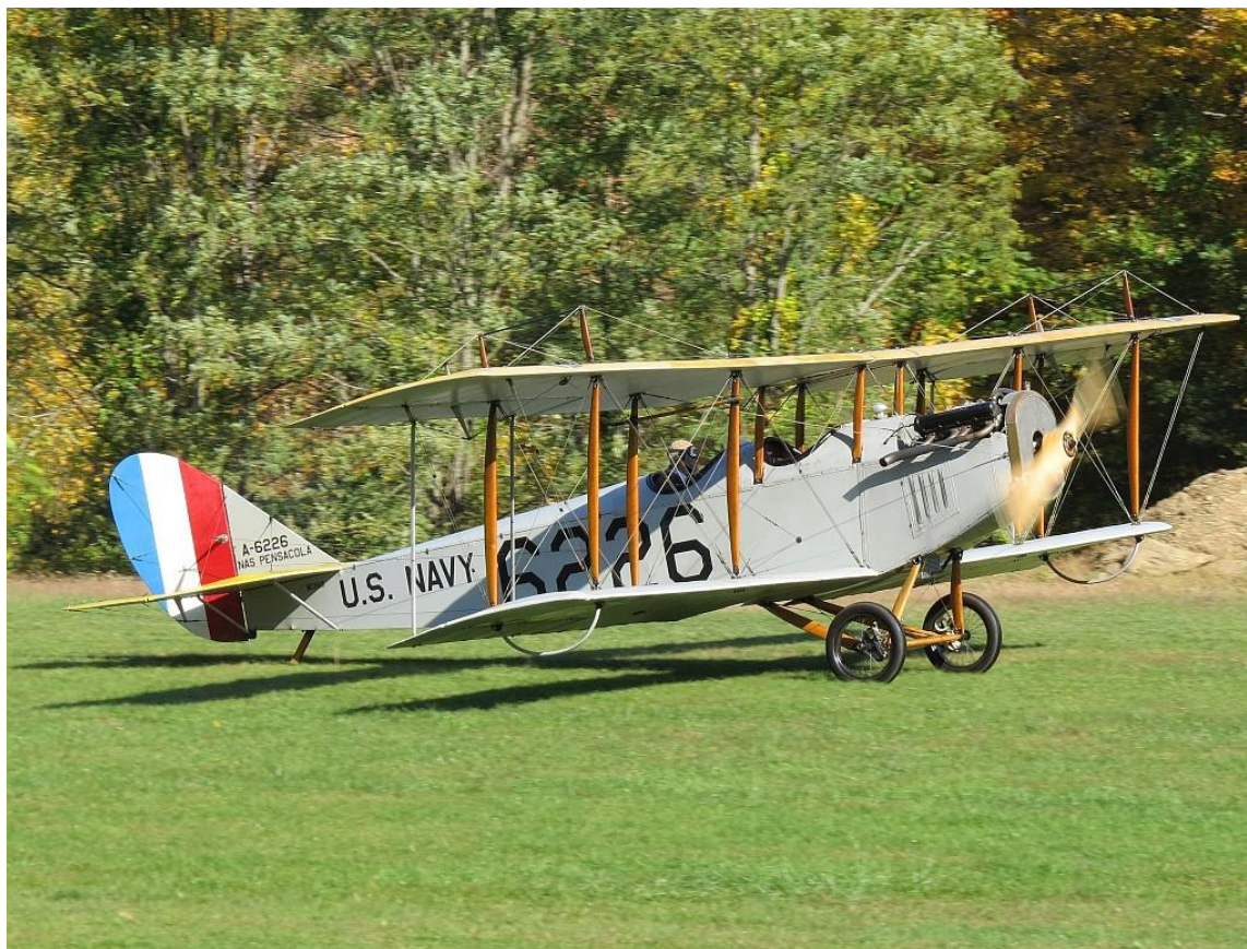
Ken Cassens taxis the Old Rhinebeck Aerodrome's 1917 Curtiss JN-4H "Jenny" following a flight demonstration of the aircraft during one of the Aerodrome's weekend airshows. The JN-4H was one of the final production versions and substituted a 150 or 180-horsepower Hispano Suiza engine for the unreliable OX-5 engine used in earlier variants of the "Jenny". The JN-4H also had strut-connected ailerons on both wings.
