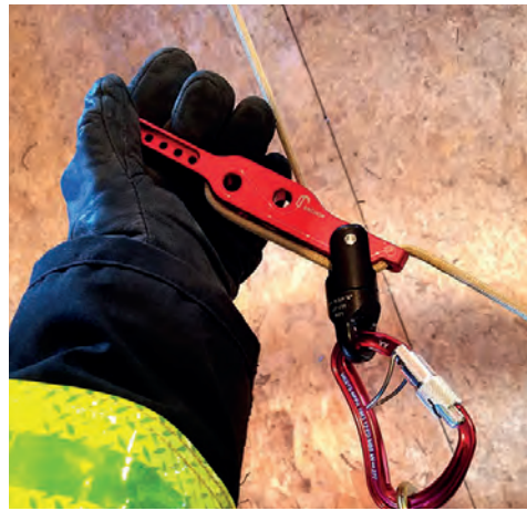
RPI's Phoenix is one of several lever-style devices (hence CMC's LEVR name for their device) where the body becomes the handle. This particular model is unique in our selection because it incorporates an integral swivel
