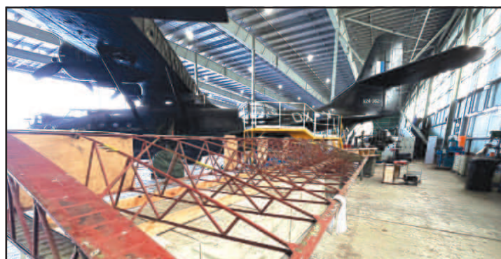
Left hand inboard trailing edge with some ribs replaced. The green ribs are ribs from NZ repaired and installed.
