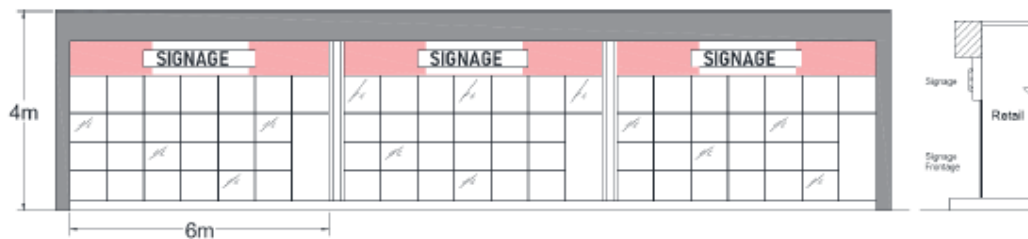
Figure 1 - Typical Retail signage- Elevation and Section
