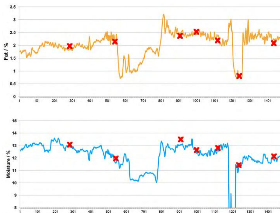
Figure 3: Comparison of real-time measurements with FT-NIR (orange: fat, blue: moisture) and laboratory measurements (red)
