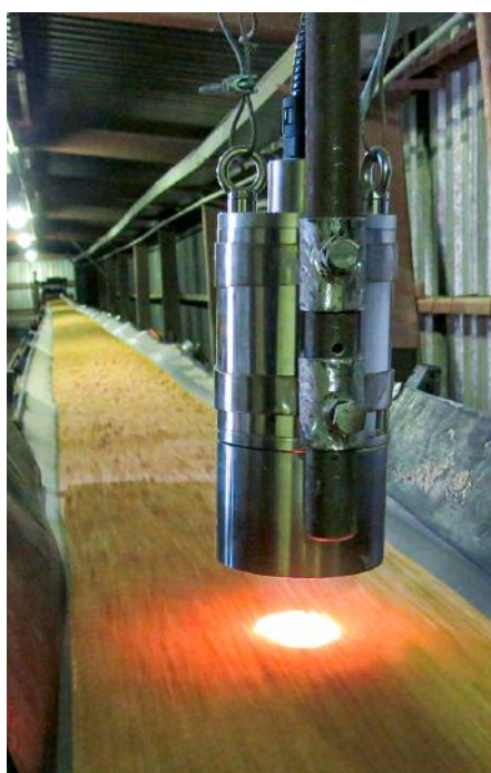
Figure 2: Test installation of an FT-NIR sensor above a conveyor belt carrying soybean meal
