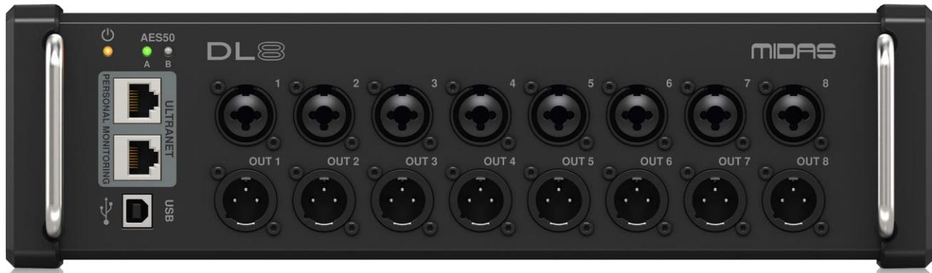
Digital mixing has revolutionized virtually everything in the live entertainment production workflow, and now that same cutting-edge technology brings live production signal distribution into the modern age. The Midas DL8 Stage Box provides 8 award-winning Midas PRO microphone preamplifiers with switchable 48 V phantom power, along with 8 electronically balanced low-impedance line-level outputs.
