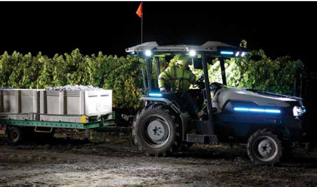
Monarch MK-V electric tractor operating in a California vineyard.
