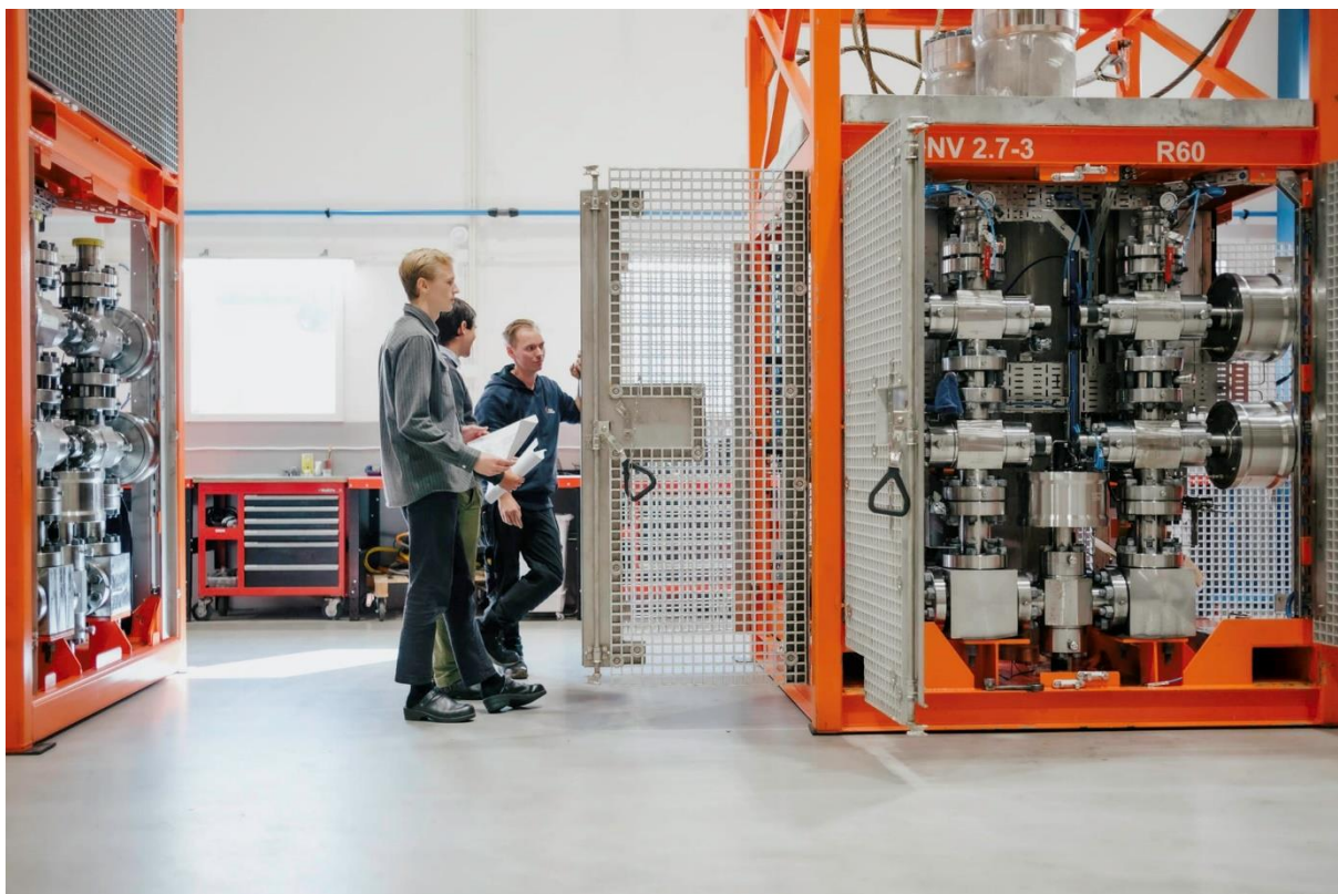
FourPhase DualFlow desander being readied in FourPhase Bergen workshop.
