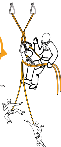
Belaying the second climber to the belaying station through a tube
