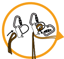
Belaying two second climbers at a belay station using a multifunctional belay device (Shuttle)
