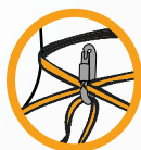
Improvised harness from a 150-cm sling If the person is unconscious, add a chest harness
