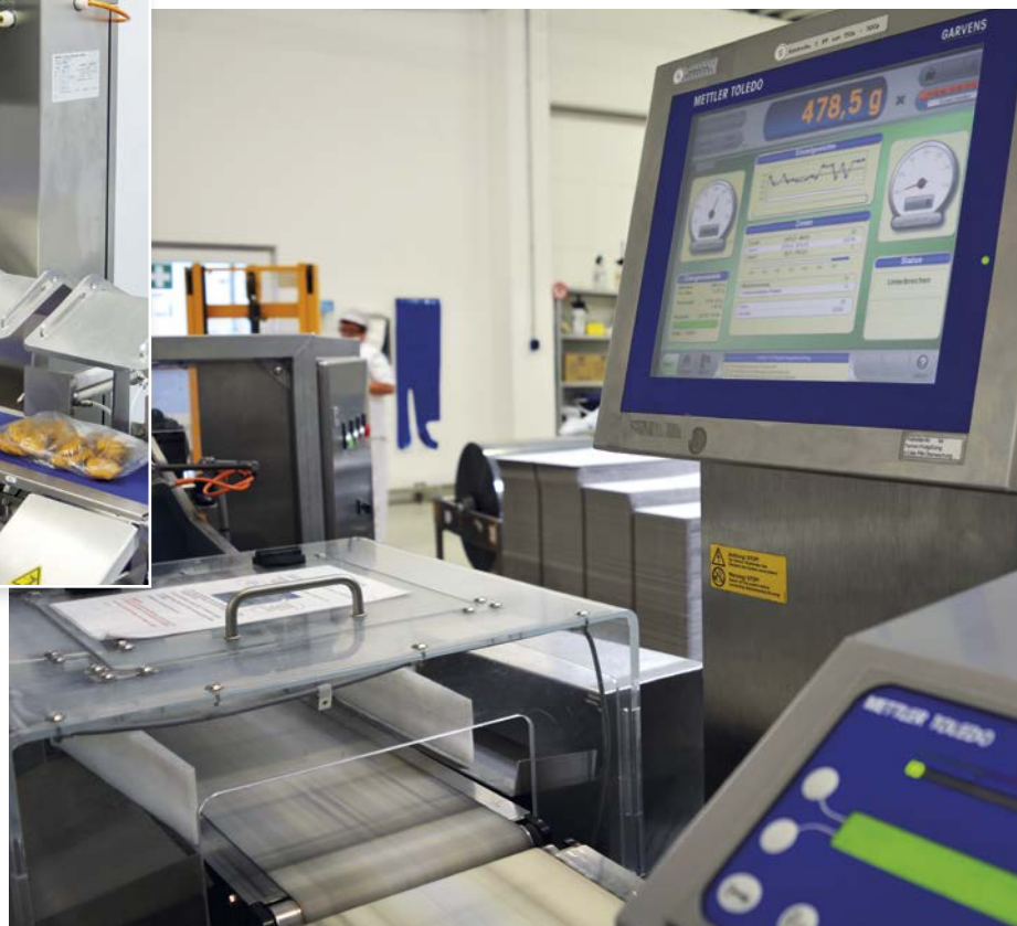
Mettler-Toledo CM (Checkweighing and Metal Detection) Washdown Combination System inspecting meat products.
