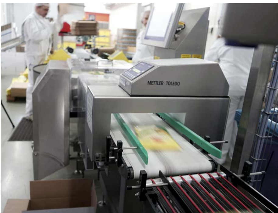
Mettler-Toledo CM (Checkweighing and Metal Detection) Combination System inspecting packs of cheese (photos: Mettler-Toledo)
