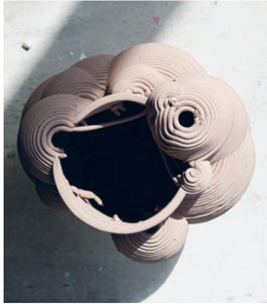
The sculptures are constructed using additive printing. Image courtesy and credit: Rafael Gil Cordeiro.
