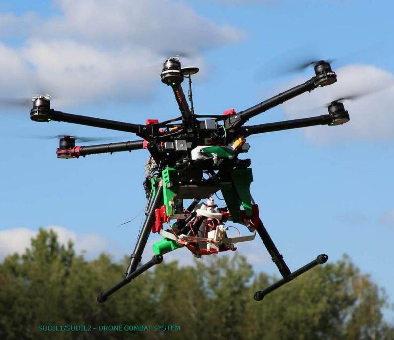
SUDIL is a second generation anti-drone platform that automatically detects and tracks an unwanted flying object. The detected intruder is intercepted using a net and towed to a safe location with the ability drop it with parachute at any time. SUDIL can be integrated with a drone detection system, thus creating a comprehensive anti-drone defense system. The platform is equipped with emergency landing systems and has its own mobile ground control station.
