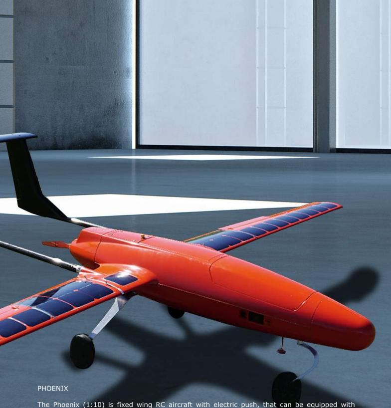
The Phoenix (1:10) is fixed wing RC aircraft with electric push, that can be equipped with photovoltaic panels. Thanks to the autopilot system, the model can perform missions in automatic, semi-automatic and manual modes. It is mainly used for testing on-board systems and for carrying various cameras. It is adapted to land mapping, in particular to obtain images of agricultural and forest areas.
