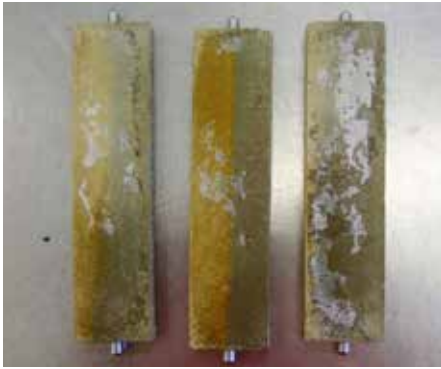
Figure 8: Intact mortar test specimens with GBS 234 at a GBS/CL ratio of 75/25 after 4,380 days at 20°C
