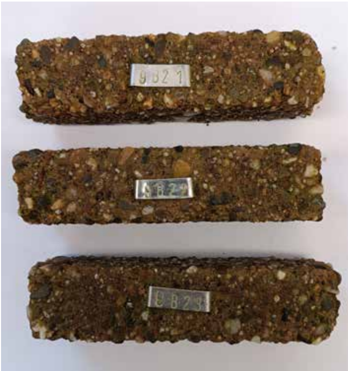
Figure 32: Mortar test specimen with Portland cement after 21 years of storage in water with lime-dissolving carbonic acid ( w/c = 0.45 , c = 320 \text{ kg/m}^3 )
