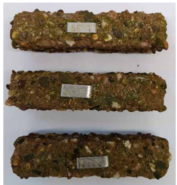
Figure 31: Mortar test specimen with Portland limestone cement after 21 years of storage in water with lime-dissolving carbonic acid (w/c = 0.70, c = 300 kg/m 3 )
