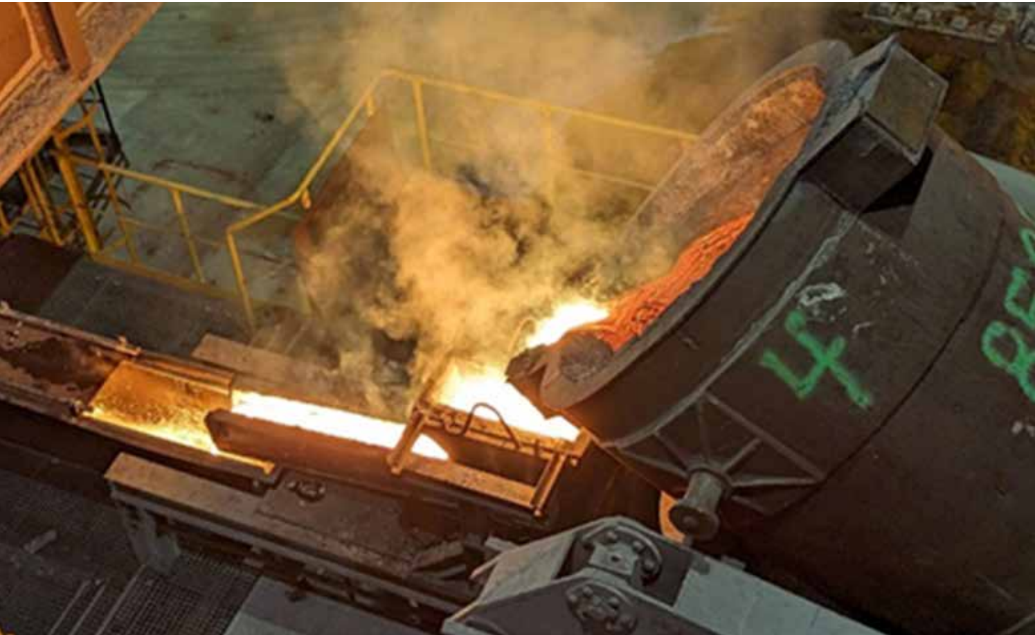
Figure 12: Water granulation of EHMS during the second large-scale campaign
