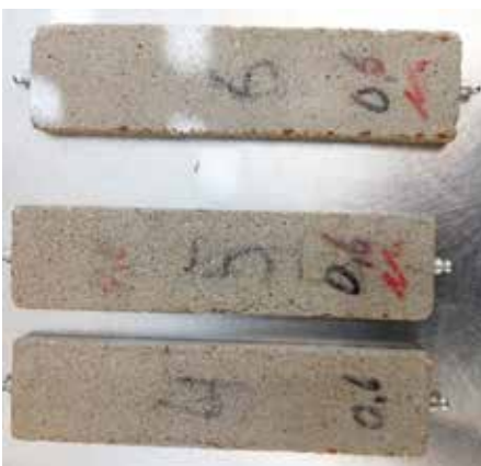
Figure 18: Mortar test specimen with Slagstar® (w/c = 0.6) after 20 years of storage at 8°C
