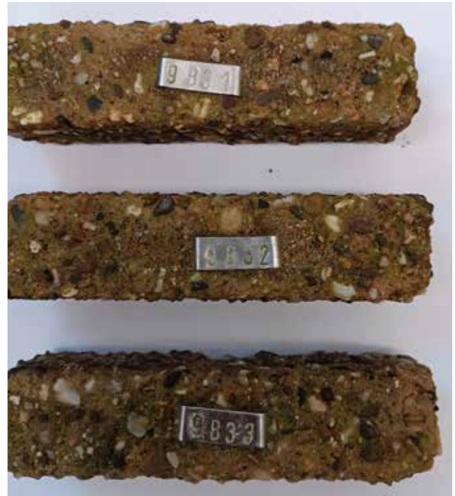
Figure 33: Mortar test specimen with Portland cement after 21 years of storage in water with lime-dissolving carbonic acid ( w/c = 0.70 , c = 300 \text{ kg/m}^3 )
