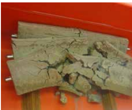
Figure 5: Destroyed mortar test specimens with GBS 234 at a GBS/CL ratio of 40/60 after 915 days at 20°C
