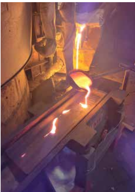
Figure 2: Pouring a ladle sample onto the copper vibrating chute (left) and removed and already cooled slag samples at the end of the blast chute (right)
