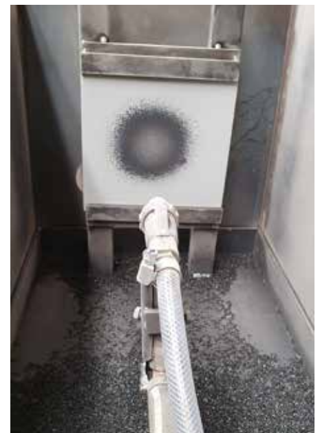
Figure 3: Positioning of the blasting gun and the blasted surface in the test box (left)
