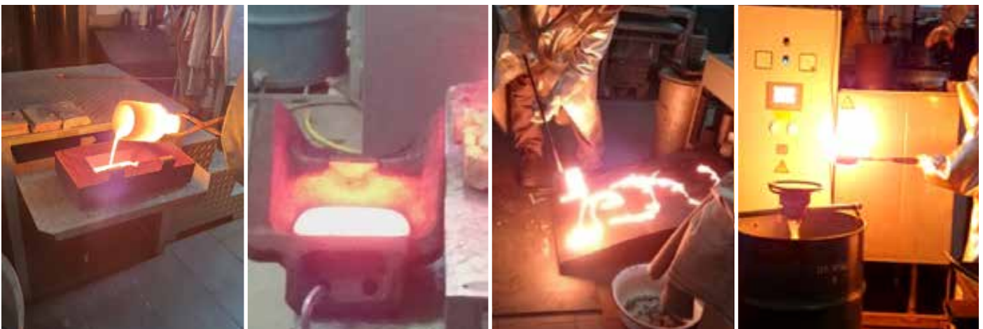
Figure 1: Tested quenching devices (from left to right): sand bed, iron mould, steel plates (uncooled), water granulation
