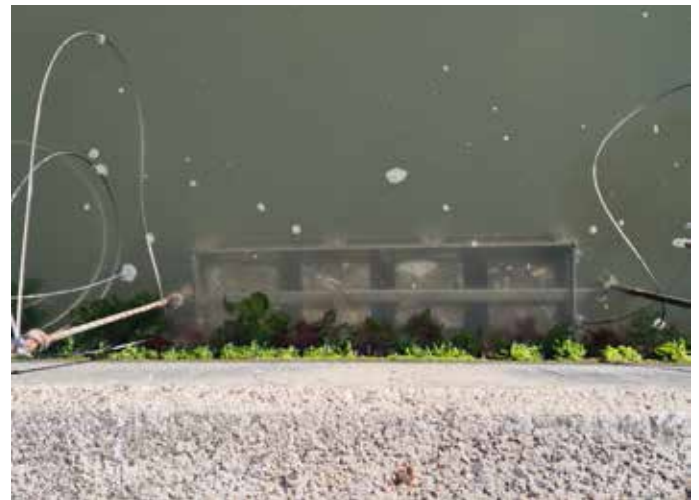
Figure 24: Storage of the concrete cubes in stainless steel cages in the water of the harbour basin
