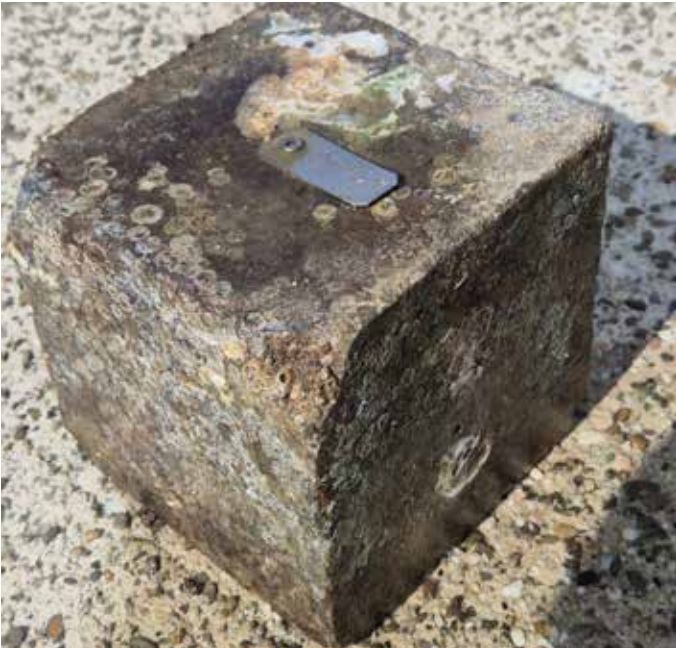
Figure 27: Corner spalling on concrete with Portland cement and MagnaDense® 20s
