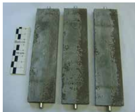
Figure 6: Intact mortar test specimens with GBS 234 at a GBS/CL ratio of 50/50 after 1,095 days at 20°C
