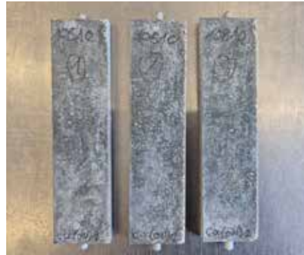
Figure 9: Intact mortar test specimens with GBS 243 at a GBS/CL ratio of 75/25 after 5,475 days at 8°C in \text{Ca(OH)}_2 solution
