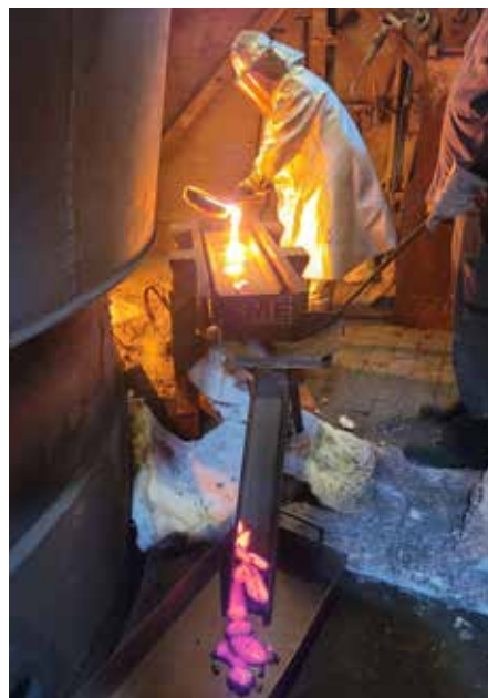
Figure 2: Pouring a ladle sample onto the copper vibrating chute (left) and removed and already cooled slag samples at the end of the blast chute (right)
