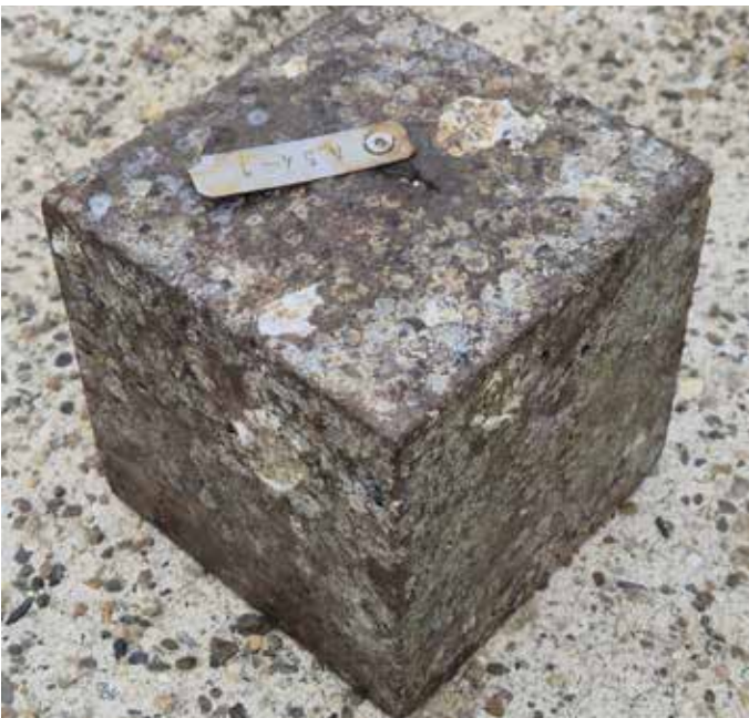
Figure 29: Intact concrete test specimen with blast furnace cement CEM III/B and EAF slag as an industrial aggregate
