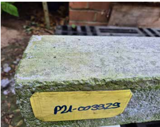
Figure 34: Intact concrete test specimen with electric furnace slag EOS-2 as an industrial aggregate after 1,392 days of outdoor storage under a roof
