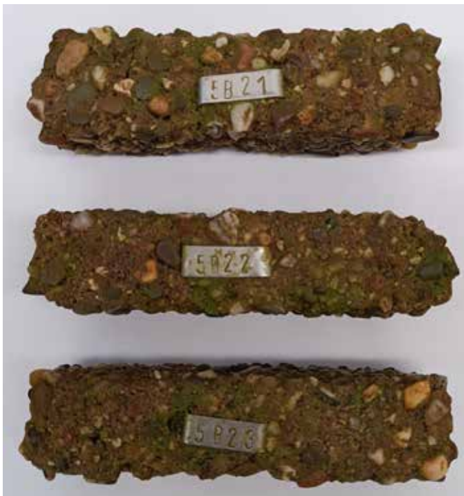
Figure 30: Mortar test specimen with Portland limestone cement after 21 years of storage in water with lime-dissolving carbonic acid (w/c = 0.45, c = 320 kg/m 3 )
