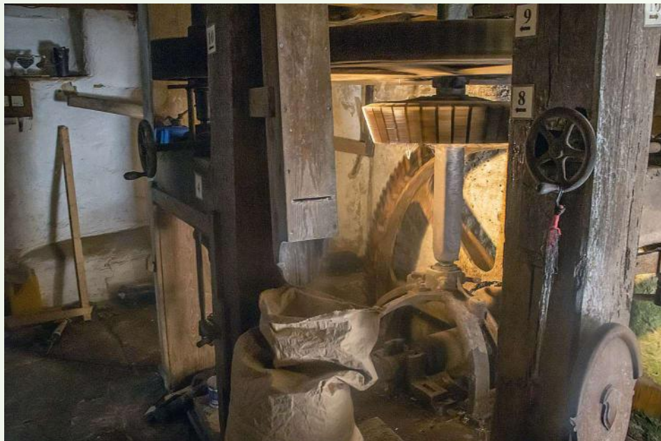
With the millstones turning, flour starts to fall down the chute into a waiting bag. Steve did explain that normally the bag is held tight against the chute to keep dust down.
