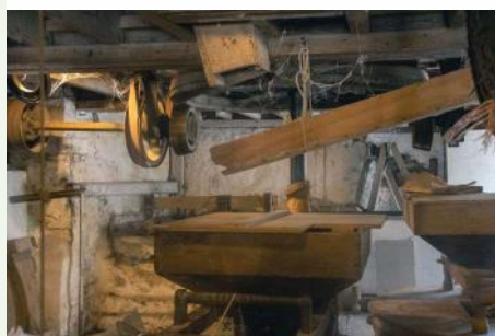
Belts, shafts and pulleys on the middle (Stone) floor.
