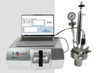
JINSP COMPANY LIMITED® RS2000 online Raman analyzer can be used for **in-situ**, **real-time and continuous online monitoring** of reaction.
