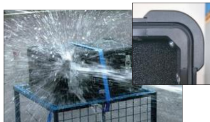
EXOcase lids have standard neoprene joints and provide IP 56 protection.
