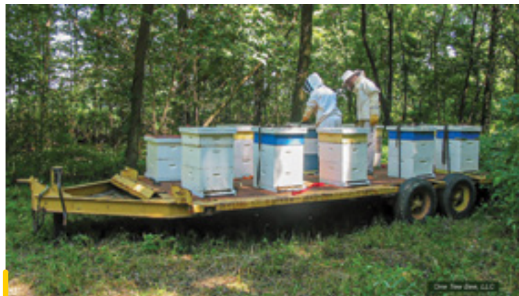
Figure 4. A heavy duty trailer with brakes and a pentel hitch on two axles.
