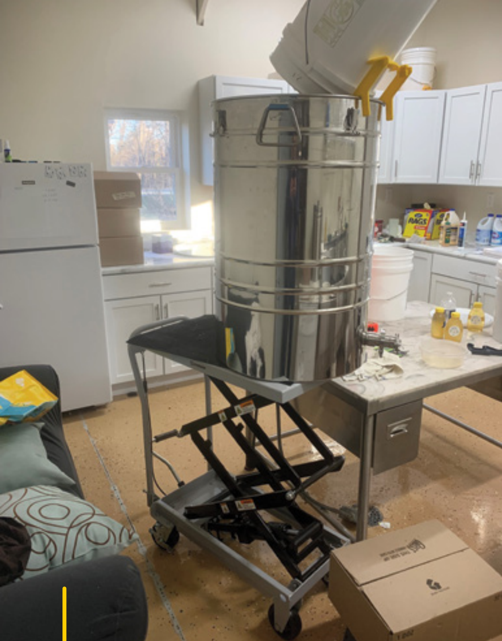
Picture 3: A 30-gallon tank on a hydraulic scissor lift was the first step to streamlining bottling. A quality stainless steel honey gate was neater than others I have tried and the high volume is enough for a day's worth of filling. With the scissor lift, I can add honey while lowered and pour when raised.
