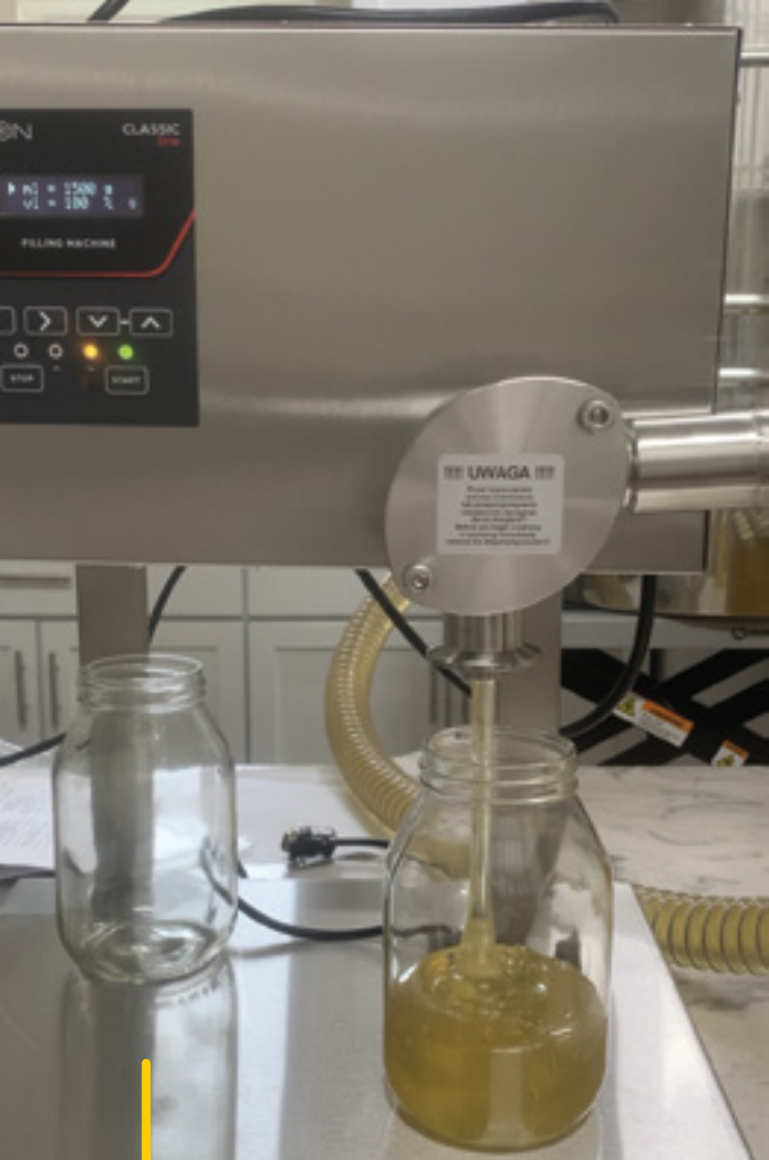
Picture 4: My latest purchase, an automatic bottler. The intake connects directly to my bottling tank. It quickly and accurately fills my jars without any drips.
