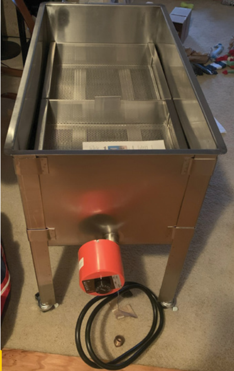
Picture 5: The heating element conversion kit of my decapping tank allows it to double as a water bath. I use it to liquefy three buckets of honey at a time. It takes about 24 hours.
