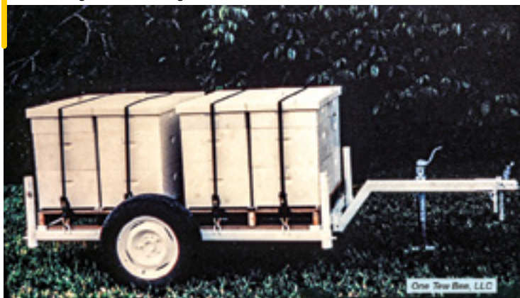
Figure 6. A custom trailer, with a detachable deck, designed to haul eight hives.
