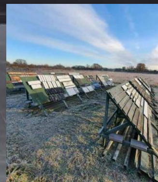
Weathering tests on our products
