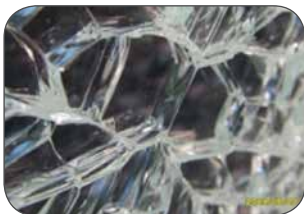
Breakage due to NiS Inclusion
