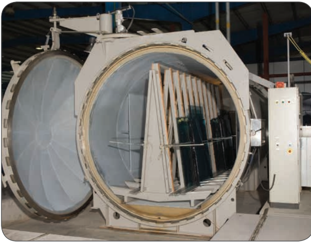
Autoclave Machine #1: Tamglass AK-3000
