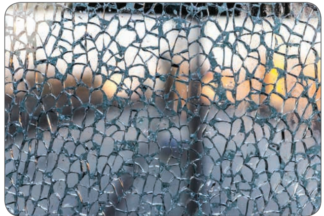
Typical Break Pattern of Tempered Glass
