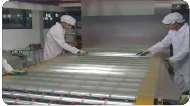
PVB or SGP Interlayer Lay-up at Lamination
