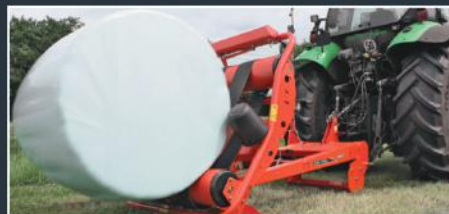
Low table height allows for gentle loading and unloading of bales
