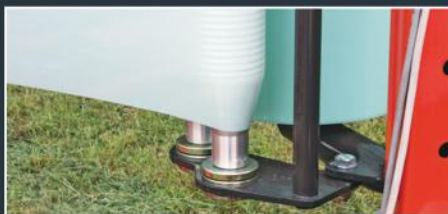
Easy film change and aluminum rollers for easy cleaning
