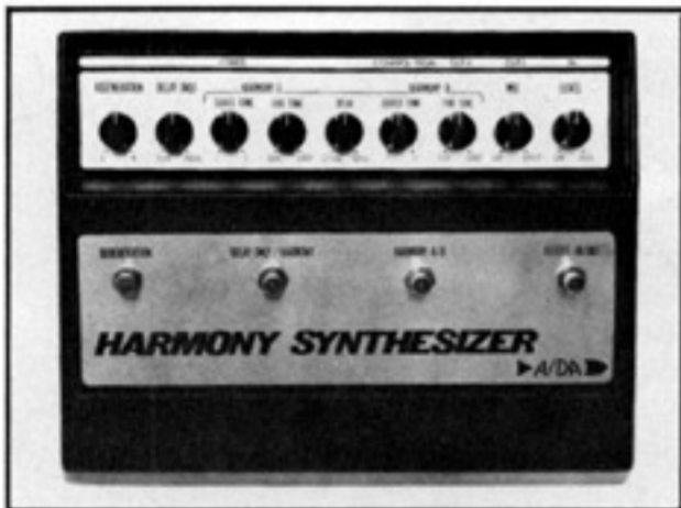
The A/DA Harmony Synthesizer shifts the pitch of single lines and chords.
