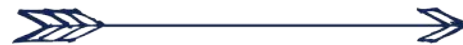
Only one style of arrow is to be used on the same item.
