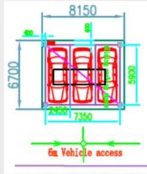
Six layers and three column lifting-sliding parking system
