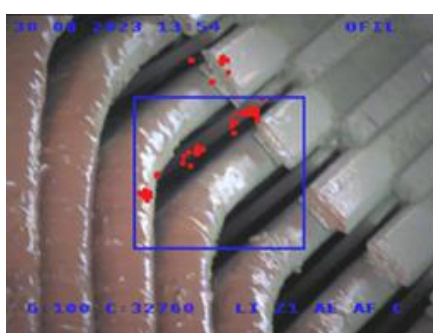
Example of PD detection on a stator during periodic maintenance
