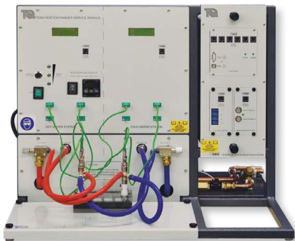
BASE UNIT FITTED WITH THE PLATE HEAT EXCHANGER AND VDAS ®
