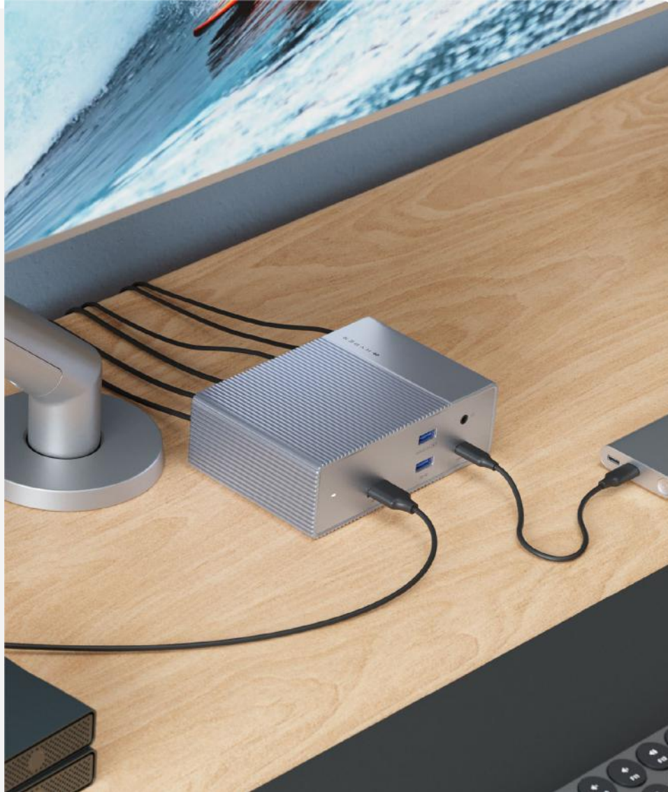
1 x Thunderbolt 3 Upstream Port 40Gbps data transfers and 85W Power Delivery.
