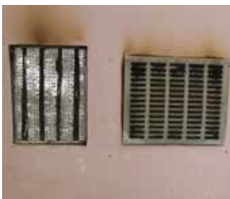
BLOCK GRILLES AFTER A FIRE TEST
