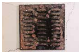
MGL Grille inside the furnace after the fire test
