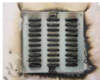
MG Grille after the fire test
