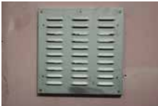
MGL Grille inside the furnace before the test
