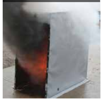
Contained fire for 45 minutes
