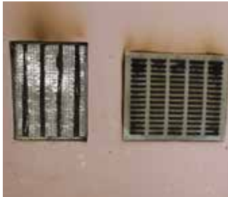
BLOCK GRILLES AFTER A FIRE TEST
