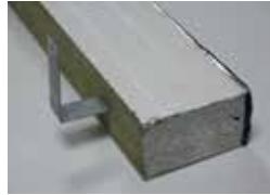
Brackets are easily pushed through the barrier
