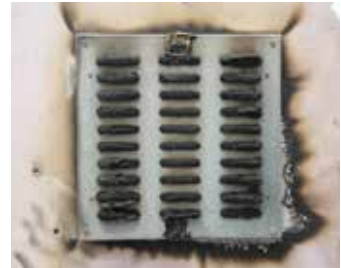
MG Grille after the fire test
