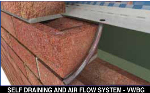
SELF DRAINING AND AIR FLOW SYSTEM - VWBG
