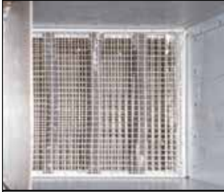
BLOCK GRILLE IN DUCTING BEFORE A FIRE TEST
