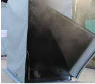
Front flap being opened to allow oxygen to enter the cover - note that fire did not reignit
