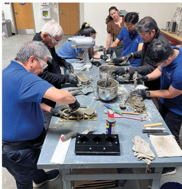
ACI Philippines Chapter representatives practicing ASTM C109/C109M mortar cube fabrication at the SoCal RC
