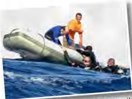
© Haitham Aziz – divers pick-up using a 4.8 metre (16 feet) length RIB equipped with a single 25 horsepower outboard engine.
