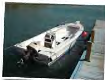
© TGI Dive Center El Gouna – a fibre glass hulled boat: 7 metre (23 feet) length equipped with a single 140 horsepower outboard engine.
